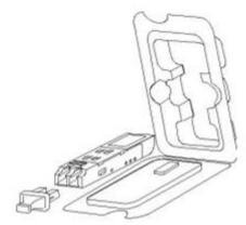
Figure 1-12. Installing the SFP Module
