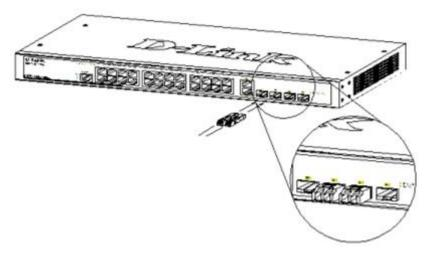
Figure 0-11. Inserting the SFP modules into the Switch
